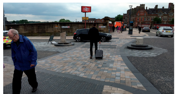
Public realm in Preston using materials as opposed to road markings to designate junctions
